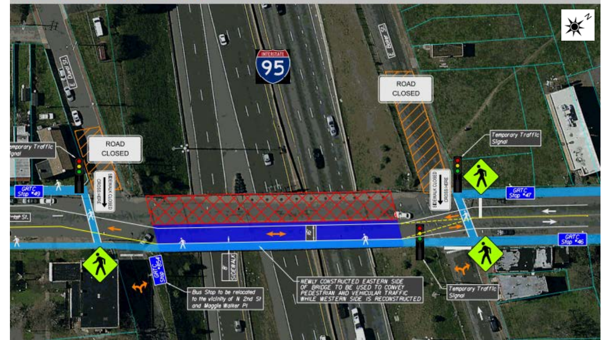
PEDESTRIAN ACCESS - SEQUENCE OF CONSTRUCTION PHASE 2 N 1st ST OVER I-95 BRIDGE REHABILITATION
